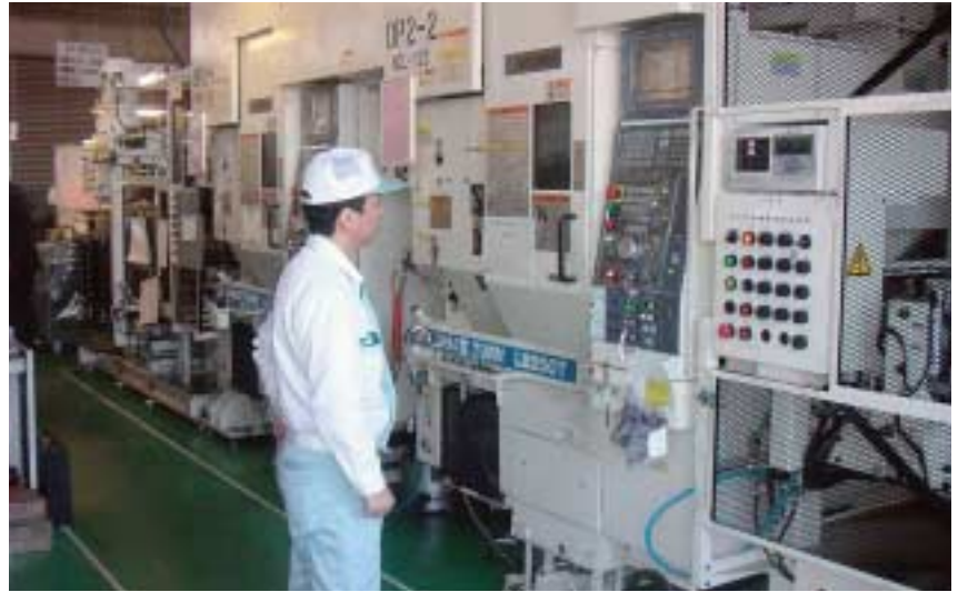
Precision turning of steering knuckles done by the SPACE TURN 250T (with loader)
